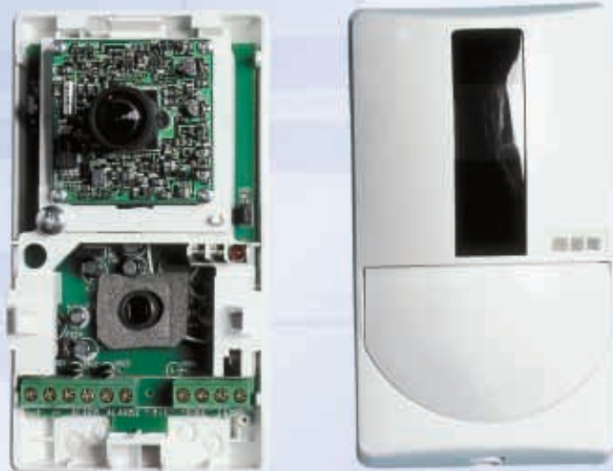
DC-20 showing miniature camera (above) and PIR sensor (below)
